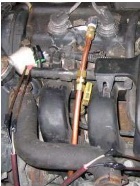
**Figure 4-15: Automobile engine compartment fire initiation device.**
