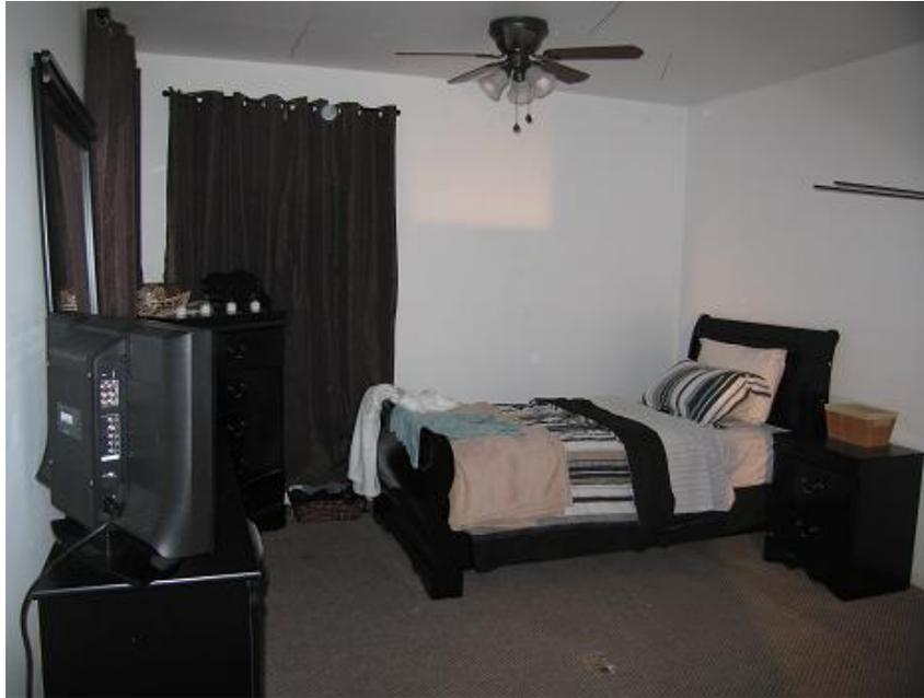
**Figure 4-4: Photograph of the furnished bedroom interior. Note the gas and particle sampling probe extending into the right side of the room at standing face level.**
