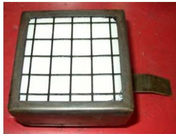
**Figure 3-3: ASTM E1354 Cone calorimeter sample holder**
